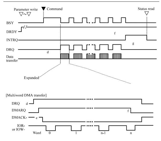
Figure 5.7 Normal DMA data transfer
