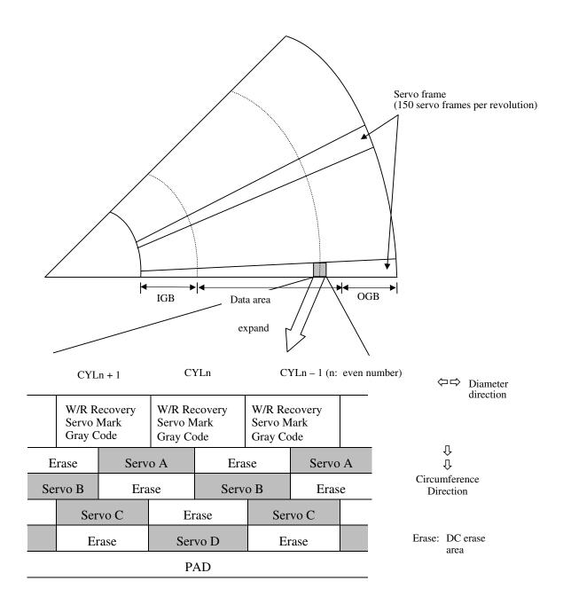
Figure 4.7 Physical sector servo configuration on disk surface
