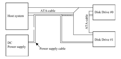
Figure 3.9 Cable connections
