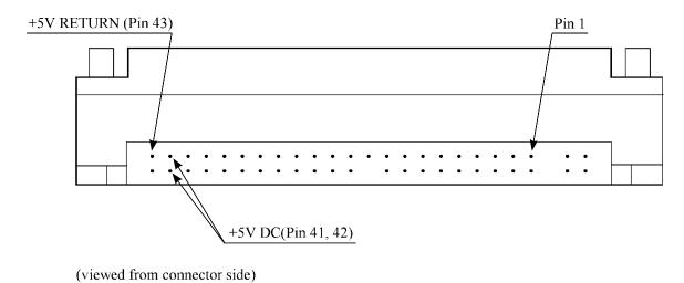
Figure 3.10 Power supply connector pins (CN1)
