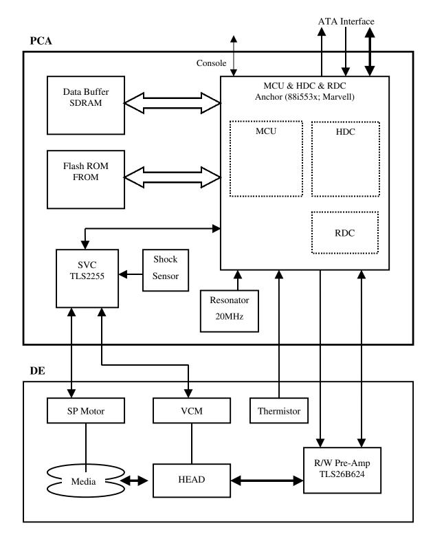
**Figure 4.2 Circuit Configuration**
