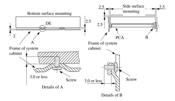
Figure 3.3 Mounting frame structure
