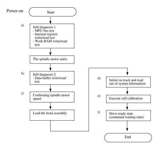
Figure 4.3 Power-on operation sequence
