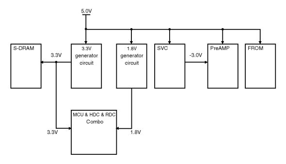
**Figure 4.1 Power Supply Configuration**
