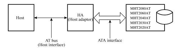
Figure 2.2 1 drive system configuration
