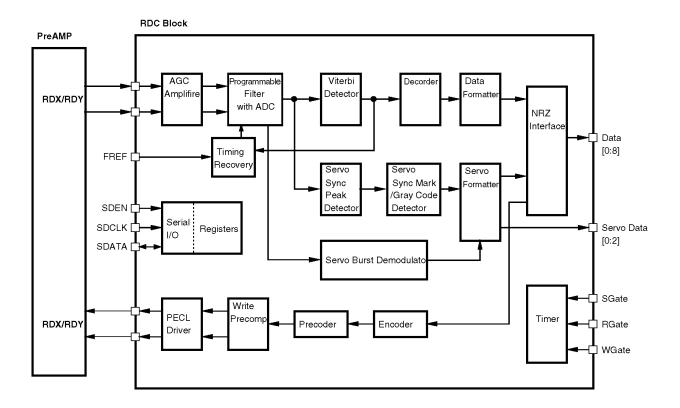
Figure 4.4 Read/write circuit block diagram
