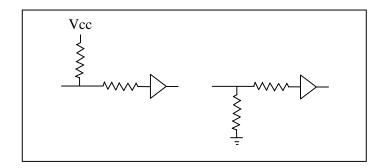
Figure 5.8 Ultra DMA termination with pull-up or pull-down
