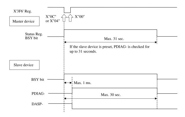
Figure 6.3 Response to software reset
