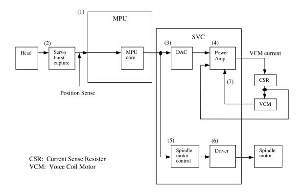
Figure 4.6 Block diagram of servo control circuit
