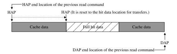
2) The read requested data is transferred, and a new read-ahead operation is not performed.
