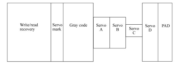
Figure 4.8 Servo frame format
