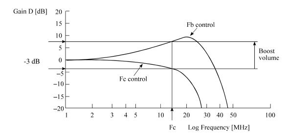
Figure 4.5 Frequency characteristic of programmable filter
