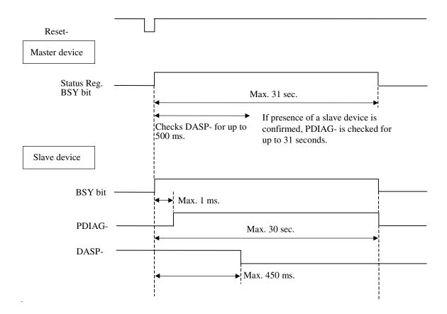
Figure 6.2 Response to hardware reset
